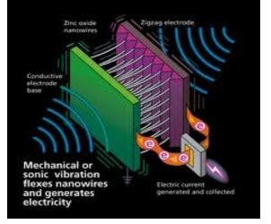
The technique essentially provides a new method of power generation; generator could be coupled with devices that are difficult or inefficient to power using conventional means. One important application is powering implantable biological sensors.
