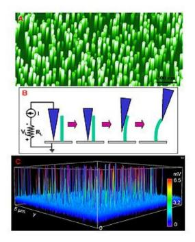
The nanowires arrays are grown using a standard vaporliquid-solid process in a small tube furnace. First, gold nanoparticles were deposited onto a sapphire substrate placed in one end of the furnace. An argon carrier gas was then flowed into the furnace as zinc oxide powder was heated. The nanowires grew beneath the gold nanoparticles, which serve as catalysts.
