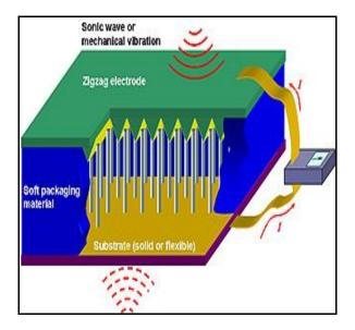
Nanogenerator allows us to harvest or recycle energy from many sources to power these devices. The electrode is then lowered on top of the nanowires array, leaving just enough space so that a significant number of the nanowires are free to flex within the gaps created by the tips. Moved by mechanical energy such as waves or vibration, the nanowires periodically contact the tips, transferring their electrical charges.
