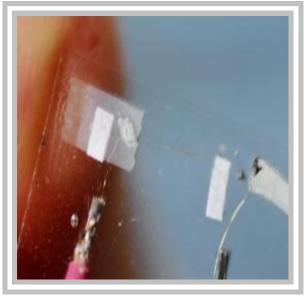
Close-up image shows a pair of entangled fibers that make up a microfiber nanogenerator. Both fibers are coated with zinc oxide nanowires; one fiber is additionally coated with gold. When rubbed together, they generate electrical current.
